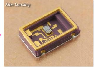
Tin is diffused and ⟨bonded⟩ Direct bonding is also possible
