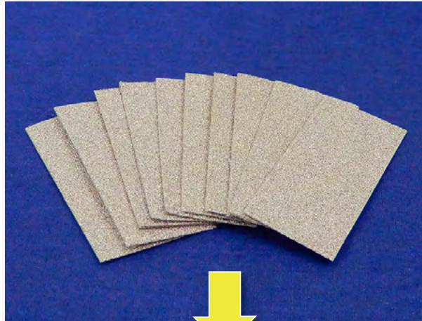
After bonding of multi-layer Nickel foam at 2 points at once
