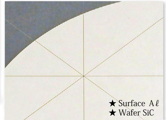
Radial full cutting of aluminum sputtered SiC wafer
