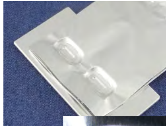
[Bonding of Al multi-layer foil and an Al plate at 2 points at once]
