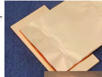
[Bonding of Cu multi-layer foil and a Cu plate at 2 points at once]
