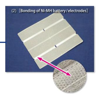
The first hybrid cars (GS450h) for LEXUS were released in Mar.2006 and Ultex's [Metal bonding technology] was adopted in assembly of these two applications.
